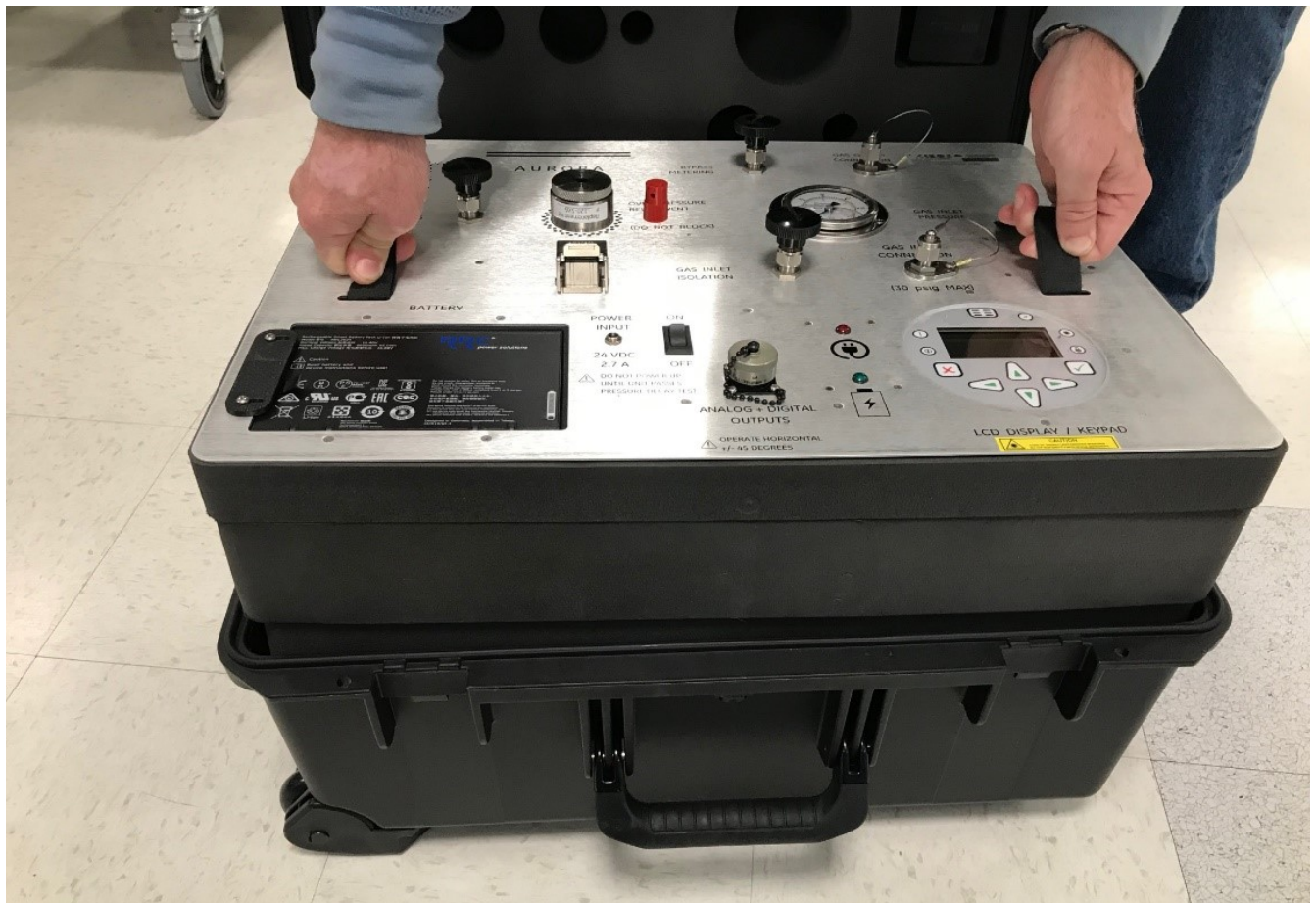
Figure 60: Replacing Inner Foam Housing into the External Pelican Case After Mirror Cleaning
