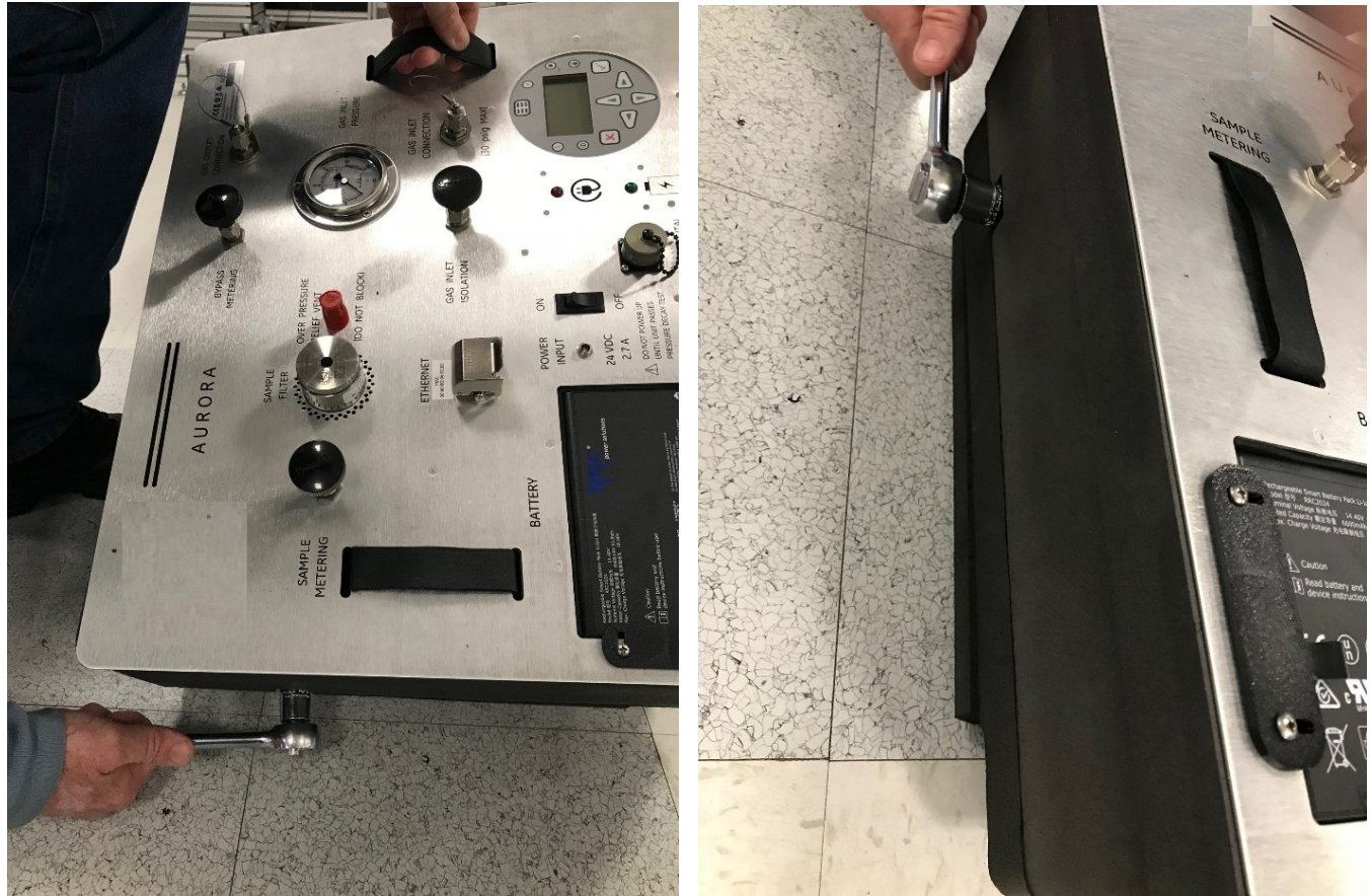
Figure 53: Extraction of Absorption Cell End Mirror from Inner Foam Housing while Holding the Assembly Upright to Prevent the Mirror from Falling out
