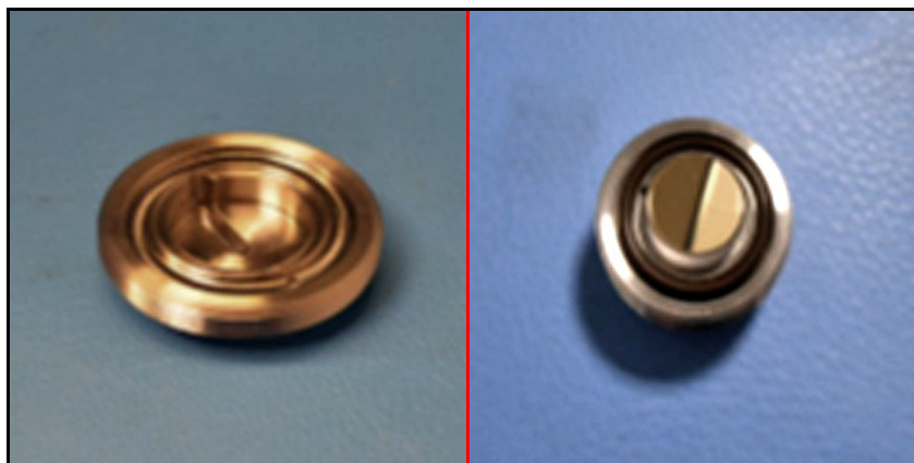
Figure 96: Replacing Cleaned Mirror into End Cap Assembly
