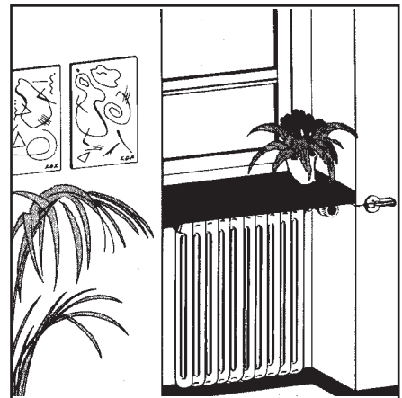
LV-4 with remote sensor. The sill creates a heat pocket; in this case a thermostat with remote sensor is necessary.
