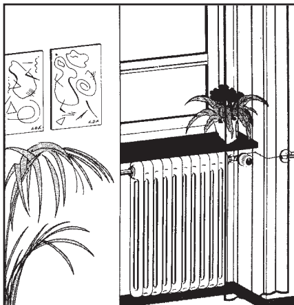
LV-4 with remote sensor. Valve is covered by a curtain; remote sensor has been mounted away from the curtain.
