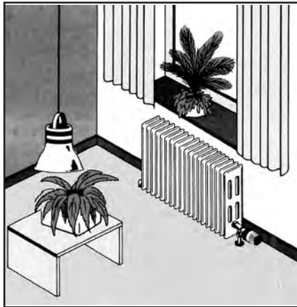
LV-4 with RV-4 reversed angle body on forced hot water radiator.
