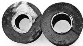
The cross section of the coil on the right shows how internal corrosion caused by improper piping, trapping and venting may destroy coils from the inside out.
