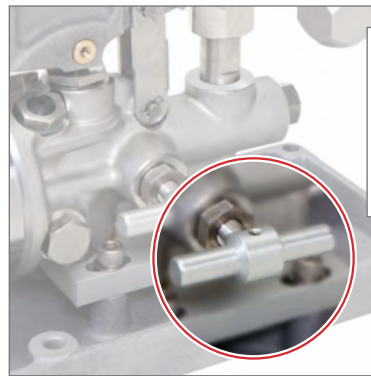
then open the vent valve.
