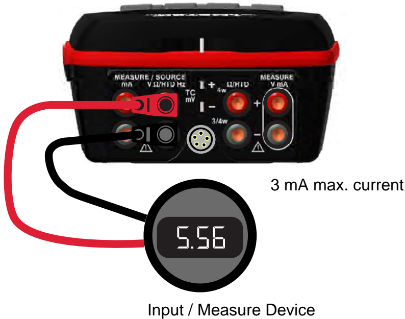
Figure 18 Connections for Testing an Output Device
