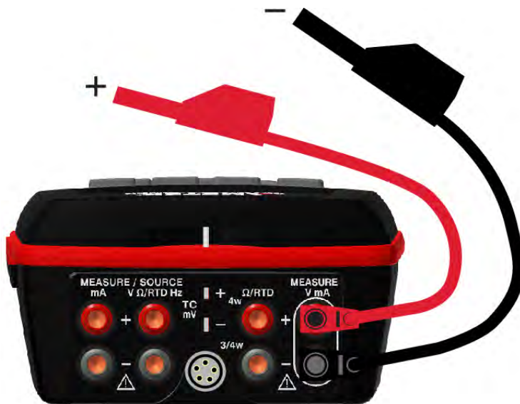
Figure 13 mA current measurement connection (upper window)
