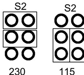
4. To change the AC configuration, remove the jumpers and place them according to the above diagram.
