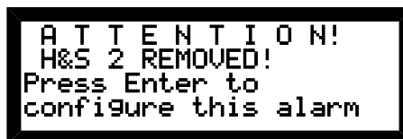
Figure 28 - Horn And Strobe Removed
