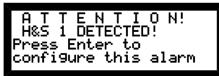
Figure 27 - Horn And Strobe Detected
