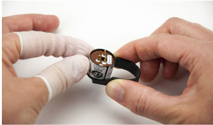
Figure 16: Using Removal Tool
