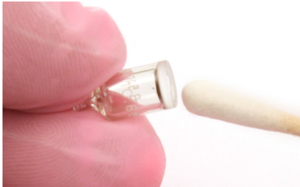
Figure 9: Polishing the Electrode Lamp Window
