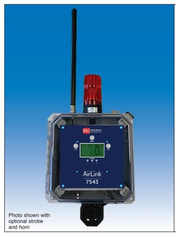
The RKI Instruments 7543 six channel gas monitor with 3 dry contact relays can monitor up to 6 individual Wireless gas detectors and transmitters. RS-485 Modbus output allows for data communication to a PLC or other system monitoring device. Available with an optional WirelessHART® module that allows the received sensor readings to be viewable on a WirelessHART® network.
