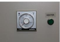
The model FTBLL12E Fluidized Temperature Bath has an easy to use dial controller for setting the bath from 100 to 1000°F. The heater light shows heater status and once flashing you allow an hour for the system to fully reach operating temperature.
