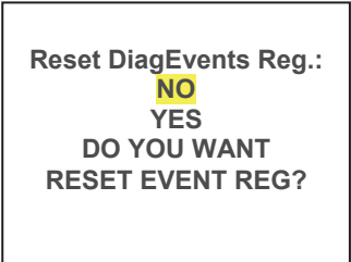
Figure 43: Resetting Diagnostic Events Register
