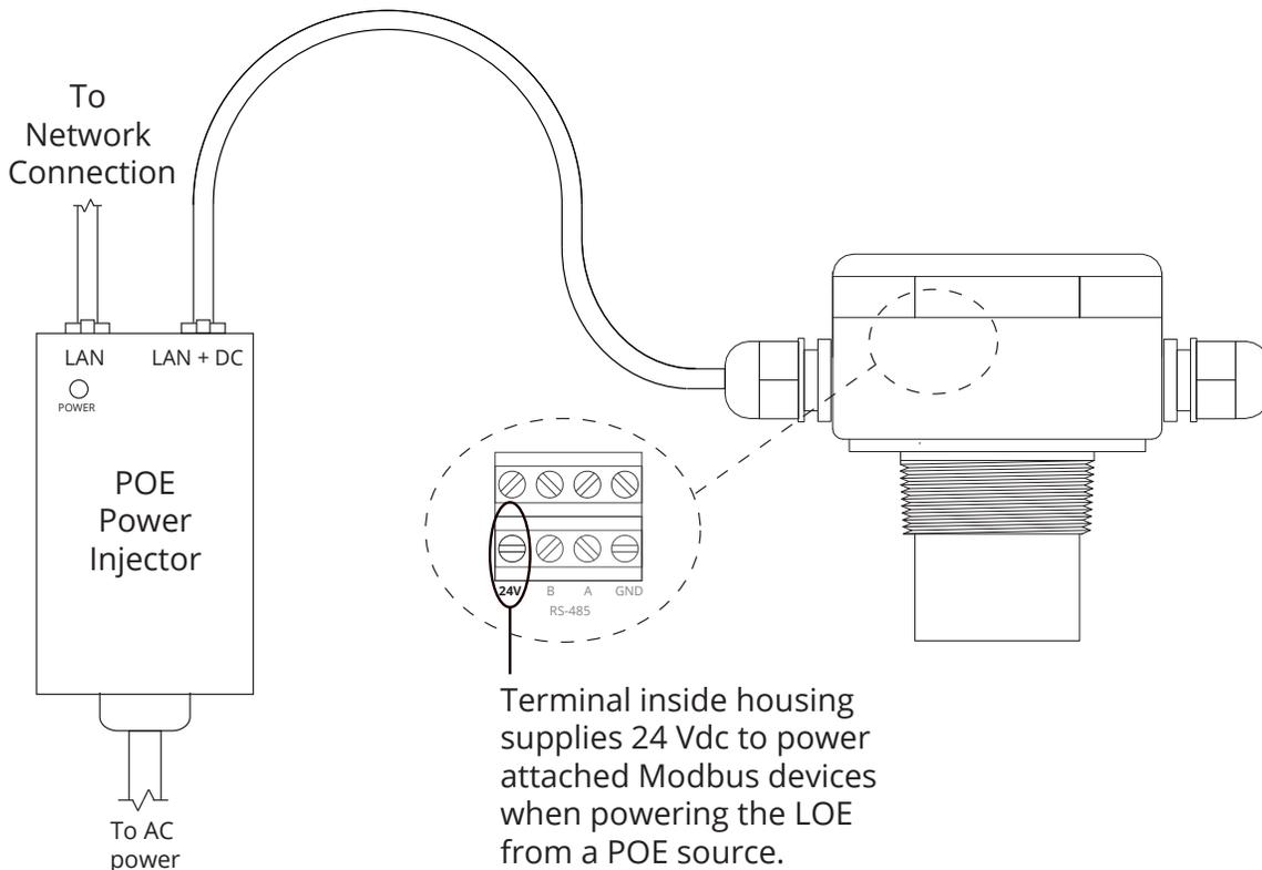
Terminal inside housing supplies 24 Vdc to power attached Modbus devices when powering the LOE from a POE source.
