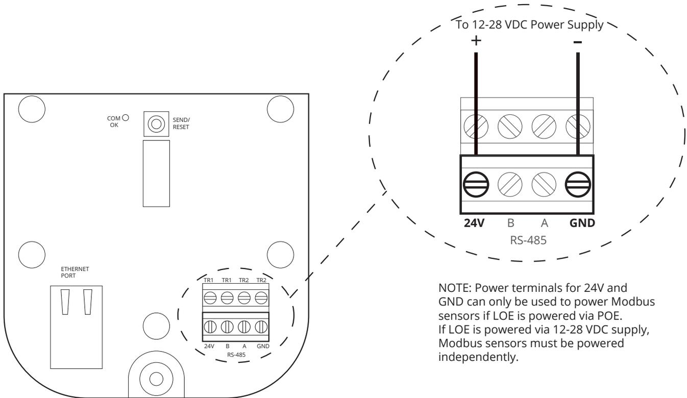
NOTE: Power terminals for 24V and GND can only be used to power Modbus sensors if LOE is powered via POE. If LOE is powered via 12-28 VDC supply, Modbus sensors must be powered independently.
