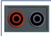
Jacks: Two standard safety banana jacks (4mm)
