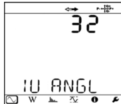
Phase angle between line current and phase voltage (3-phase 3-wire \Delta balanced)
