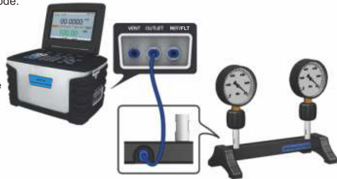
Figure 3-16 Calibrating pressure gauges
