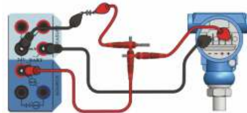
Figure 3-14 Internal series resistor and external loop power supply
