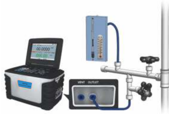
Figure 5-2 Calibrating a mercurial barometer
