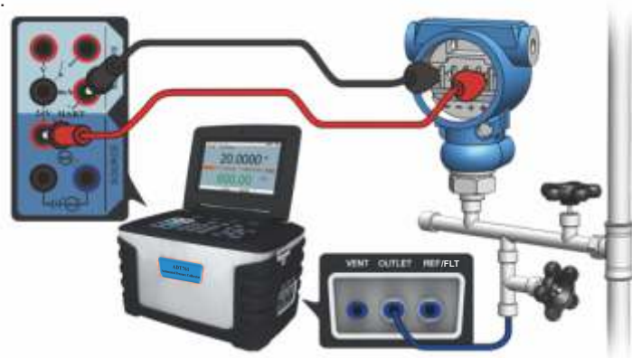
Figure 3-17 Calibrating a pressure transmitter
