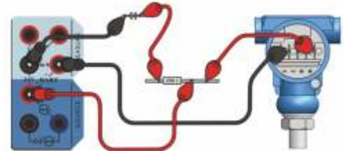
Figure 3-15 External series resistor and external loop power supply
