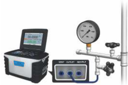
Figure 3-20 Calibrating a dial pressure gauge
