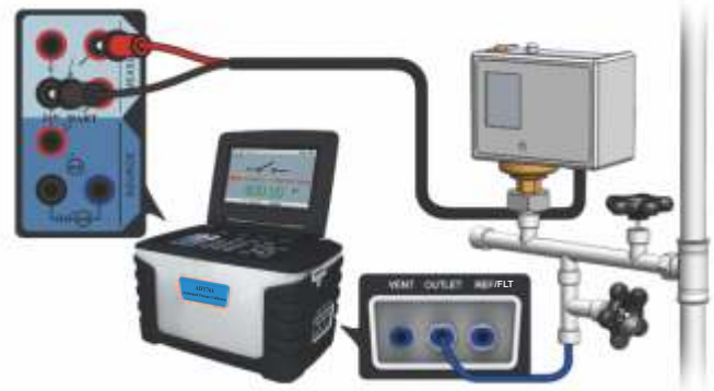
Figure 3-18 Calibrating a pressure switch
