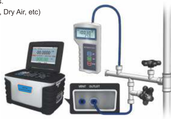
Figure 5-1 Calibrating a digital barometer
