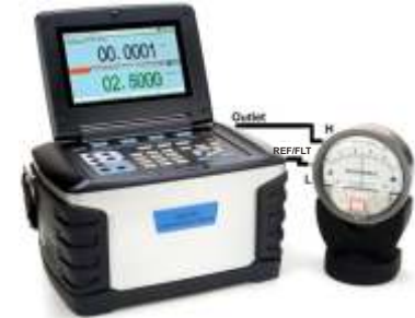
Figure 3-4 Differential pressure source
