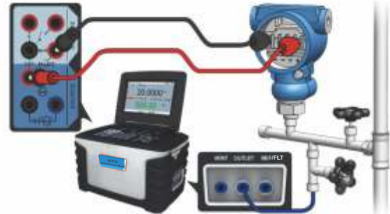
Figure 3-22 Calibrating a two-wire pressure transmitter
