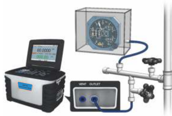
Figure 5-4 Calibrating a barometer altimeter
