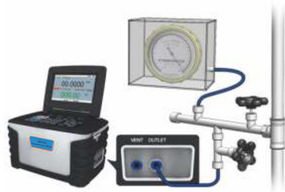
Figure 5-3 Calibrating an aneroid barometer
