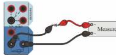
Figure 3-7 External power supply
