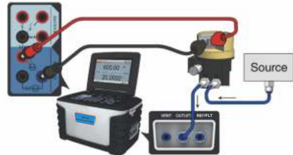
Figure 3-24 Calibrating an I/P converter
