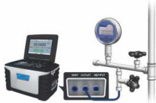
Figure 3-21 Calibrating a digital pressure gauge
