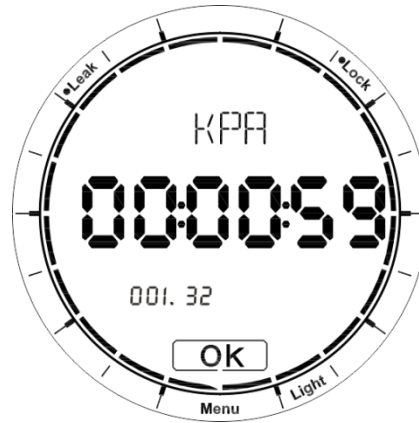
Figure7 Pressure leak test operation interface
