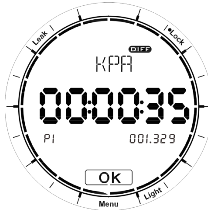
Figure 8 Pressure leak test finish interface
