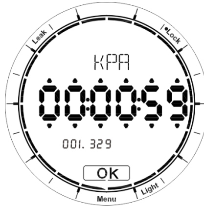
Figure 6 Pressure leak test setting interface
