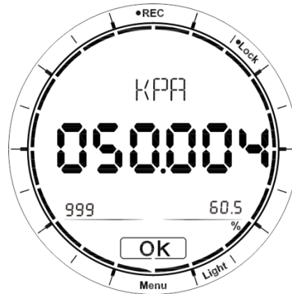
Figure 10 pressure record operation interface
