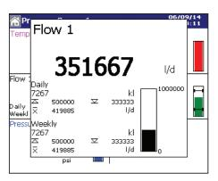
Alternatively, each totalizer can be set to reset at different intervals, for example, one resetting daily while the other resets on a weekly basis.
