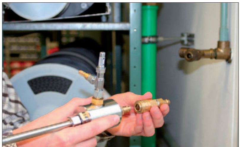
Connection of trace humidity probe testo 6651 via measurement chamber and protective filter
