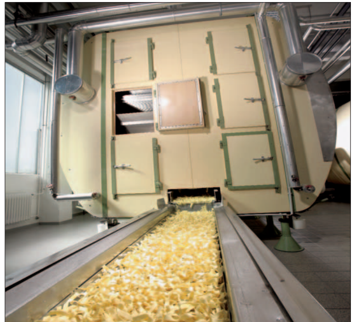
Pasta drying is carried out by measuring humidity
