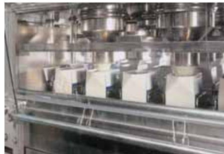
Positive pressure in the filling room maintains the hygiene conditions during filling operations in the food and pharmaceutical industry
