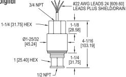
The SERIES 636 Pressure Transmitter is a low cost, fixed range, stainless steel transmitter with ±0.30% accuracy. It is designed to continuously measure pressure for years in even the toughest environmental and media conditions. Transmitters are explosion-proof, (FM approved) and meet NACE standards for off-shore applications.
