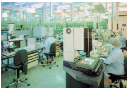
Defined pressure differences between cleanroom and adjoining rooms assure quality
