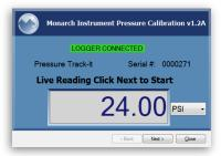
**Track-It™ Pressure Calibration Software** is a software Wizard, it automatically prompts you through the step-by-step procedure to perform your calibration.
