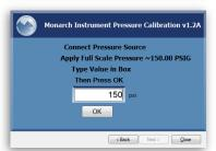
The software detects the full scale value and asks for a pressure source to be applied at that approximate value.
