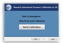
The final calibration point is the low value of the range. Wait for a stable low value and press "Send Calibration". This completes the procedure.
