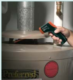
Measure temperature in hard to reach areas
