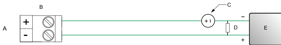
Figure 3-9: Discrete Output wiring (externally powered)
