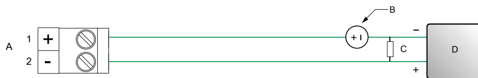
Figure 3-8: Channel B mA output wiring (externally powered)
