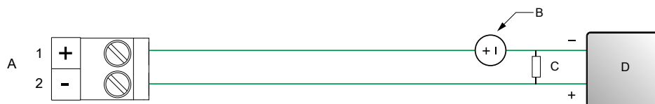
Figure 3-7: Channel A mA/HART output wiring (externally powered)
