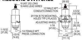
The SERIES 1000E has the same rugged construction as used in Series 1000W plus explosion-proof design are combined in this new unit. UL listed for Class I, Groups A, B, C & D; Class II, Groups E, F & G. Bellville spring movement permits mounting of control in any position and helps prevent contact chatter. High over-pressure protection and vibration resistance are also featured.
